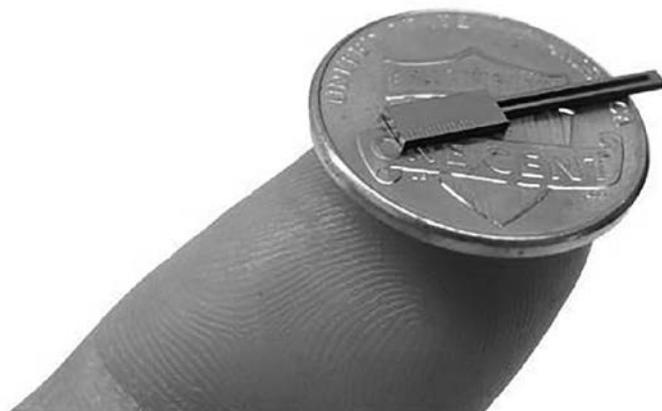
**FIGURE 11.18** MEMS-based integrated Coriolis system. (Courtesy: Integrated Sensing Systems.)
