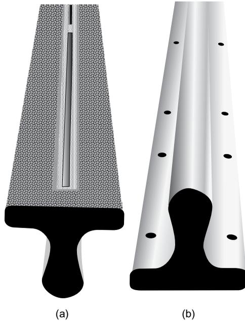
**FIGURE 6.39** (a) The impact (high ( $P_H$ )) pressure is measured with frontal slots whilst (b) the stagnation (low ( $P_L$ )) pressure is measured with sensing ports located in the stagnation zones at the rear of the sensor. (Courtesy: Emerson.)
