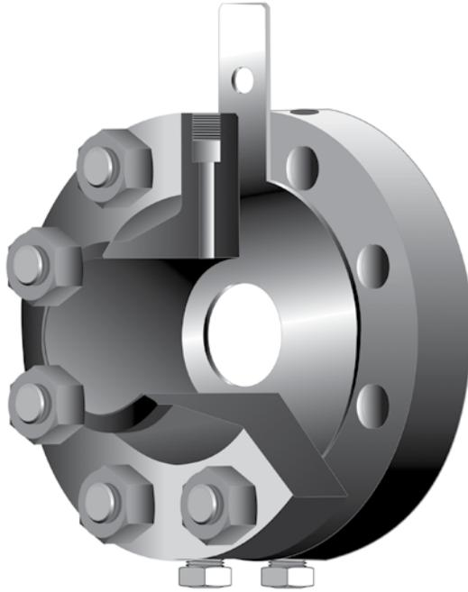
**FIGURE 6.16** Typical flange and plate assembly supplied by the manufacturer, incorporating the drilled pressure tappings.
