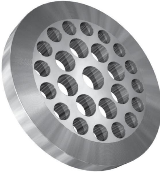
**FIGURE 4.19** CPA 50E flow conditioner comprises a steel plate,  $0.125D$ – $0.15D$  in thickness, having a central circular hole and two rings of circular holes in concentric circles around it. (Courtesy: Canada Pipeline Accessories.)
