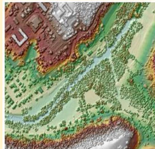
Hillshaded representations of a first return surface, or DSM, on the left and a bare earth model, or DEM, on the right.
