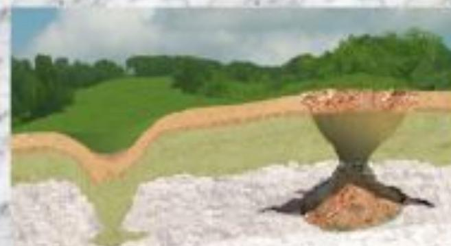
Dry sinkhole formed by slumping of cover into an ancient buried solution sink.
