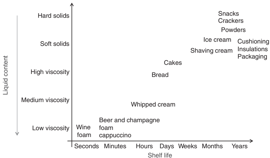
Figure 9.38 Relationship between mechanical properties of foams and their shelf-lives.
