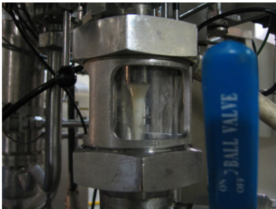
Figure 9.24 A 38% dry solids milk protein concentrate exiting a high solids vacuum evaporation unit. Source: Reproduced with permission of Clextal, France.
