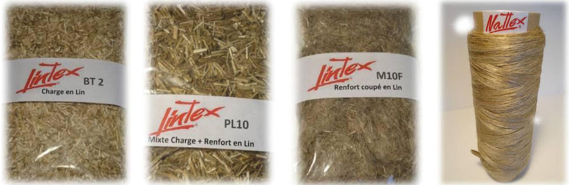
Figure 4.28 Different grades of technical flax fibers. Source: FiMaLin ® , 2011. Reproduced with permission of Dehondt Technologies.
