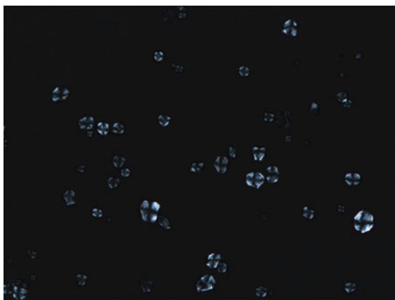
Figure 7.1 Optical microscopy of corn starch granules under polarized light (courtesy of O.H. Campanella, Purdue University, USA).
