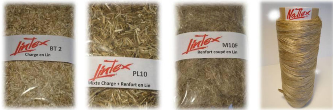
Figure 4.28 Different grades of technical flax fibers. Source: FiMaLin ® , 2011. Reproduced with permission of Dehondt Technologies. For color detail, please see color plate section.
