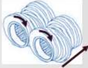
Monolobe kneading blocks, right-handed
