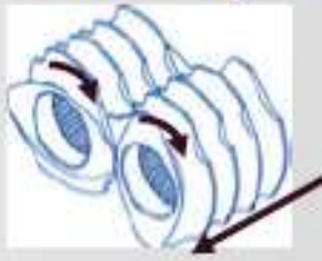
Conjugated, double flight, left-handed pitch
