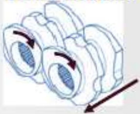
Conjugated, single flight, left-handed pitch
