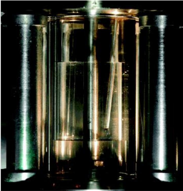
**Figure 3.** Vapor-liquid-liquid equilibrium for the ethane-methanol system.
