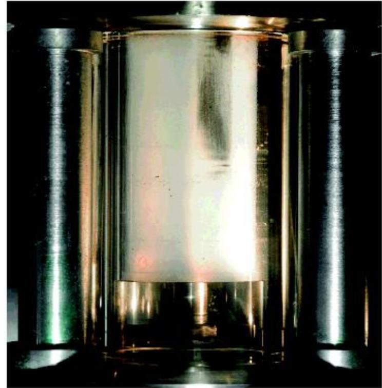
**Figure 4.** Critical opalescence observed at the upper critical end point for the ethane-methanol system.
